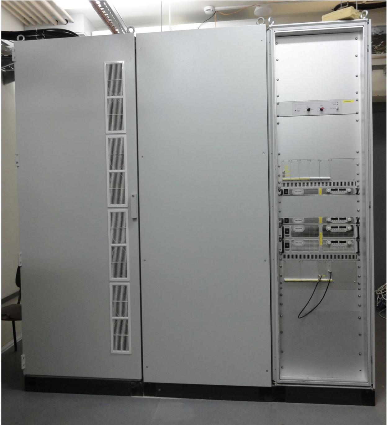
Klystron modulator and power supply rack No2 with electron gun modulator, klystron driver and power supply units of the klystron electromagnet
