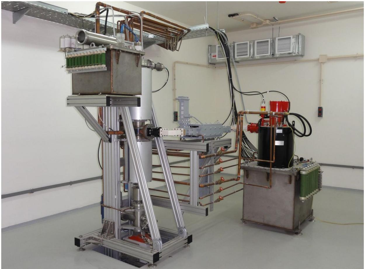
Irradiator and klystron with pulse transformer
